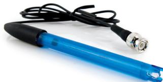
The Vernier Gel-Filled Combination pH Electrode is designed to be used with the Vernier Electrode Amplifier (order code EA-BTA) to make measurements in the pH range of 0 to 14. Our pH Electrode can be used for any lab or demonstration that can be done with a traditional pH meter, including acid-base titrations, monitoring pH in an aquarium, and investigating the water quality of streams and lakes.
